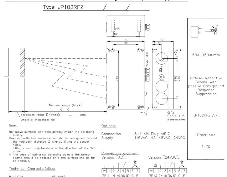
Weight approx. 3000g Protection mode **IP65** Connection terminal strip 230VAC/6VA Supply Relay 250VAC/8A, Output 1500VA, 1xCh, R Optocoupler, 60V/60mA, e1 Signal mode bright-/darkswitching, selectable 850...880nm, invisible Transmitter light \$\(\frac{1}{4}\) Steady light resist. >80kLx Interference suppress. Force synchronization (14.05.1 (03.05.1 30.04.2 <12ms/switch transition Access time Switching rate 10/s Switch indicator Level indicator LED green 4x LED red (DIANA, i) -25...+60°C
